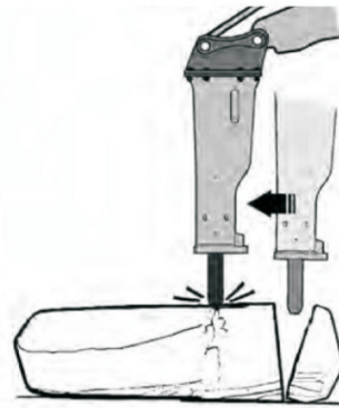
Start at the edge and work toward center.
